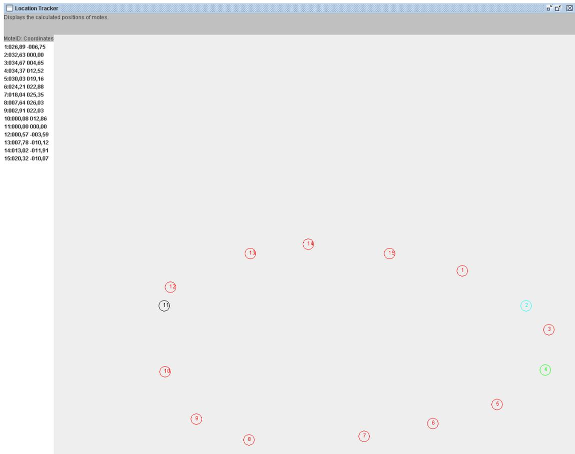
Figure 14: Calculated positions of real experiment with 15 motes in a circle
